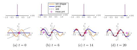
Fig. 2: Time series snap-shots of cart double pendulum actively sampling and estimating the shape underneath. The uncertainty (dashed gray lines) calculated from the collected data set drives the exploratory motion of the cart double pendulum while our method ensures that the cart double pendulum is maintained in its upright equilibrium state.
